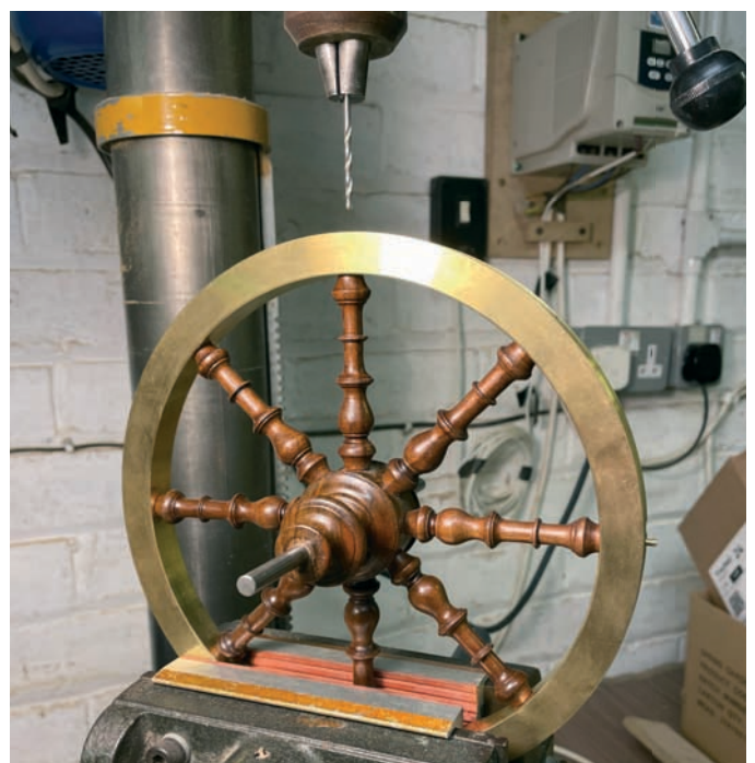
4. Drilling rim holes
