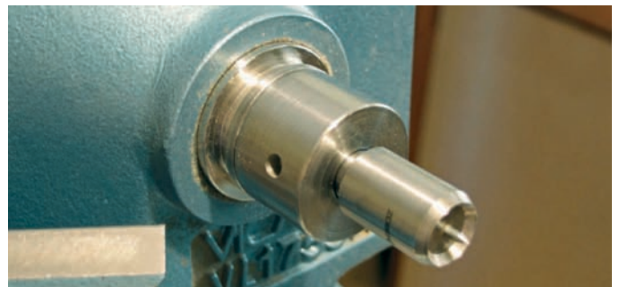
Photo 3. shows the job completed. The stub arbor is 1" in diameter which allows a tapered circular rim of 7/8" diameter, to be in contact with the wood. The tool rest needs
