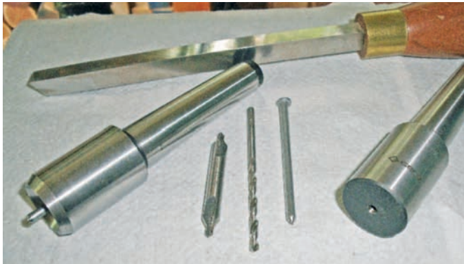
Photo 1. shows the tools I used in the making, including a suitable drill bit for the size of pin. I used a masonry nail to make the pin. With a 1/8" bit in the tailstock chuck I drilled
