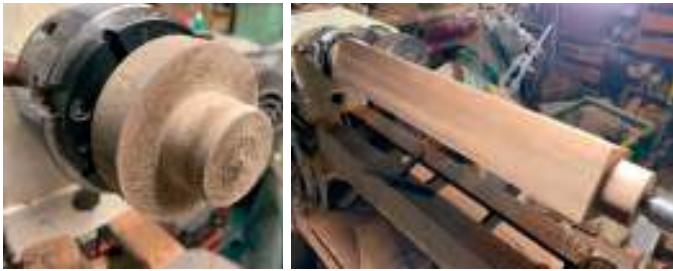
Friction drive and section B mounted showing tenon Y
