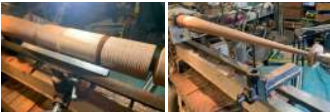
Spiky bit A - measured out to cut the grooves down to reducing diameters of taper
