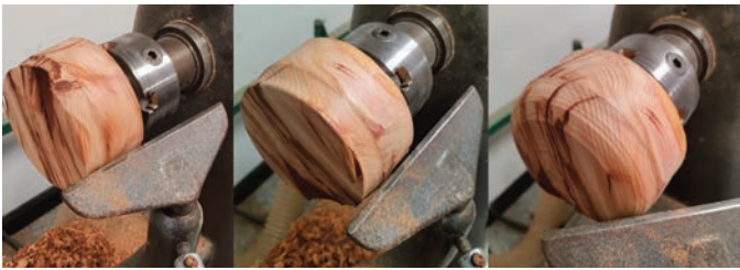
9. The piece with the imperfections removed.
