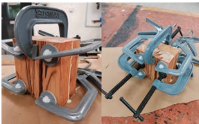
3. The gluing setup of the two square pieces.
