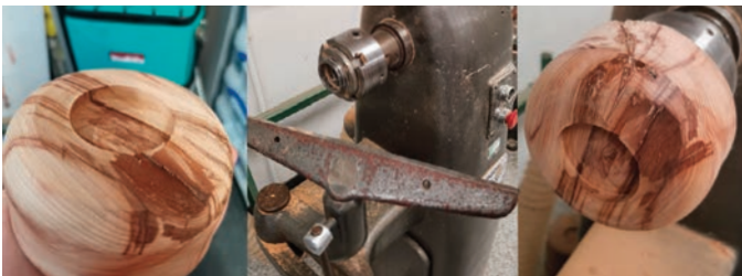
11. The final chuck attachment point.
