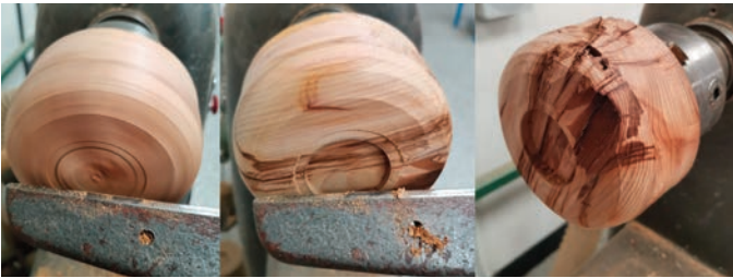
10. Creating the chucking point.
