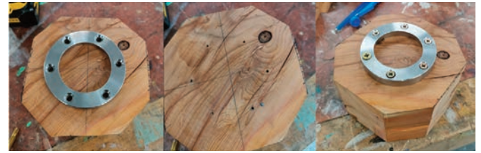
6. Attaching the faceplate
