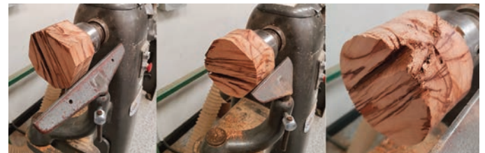
7. Turning the hexagonal piece round.
