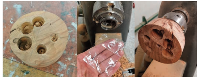
13. Mounting back on the chuck.
