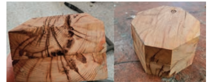
5. The hexagonal block ready to be turned.
