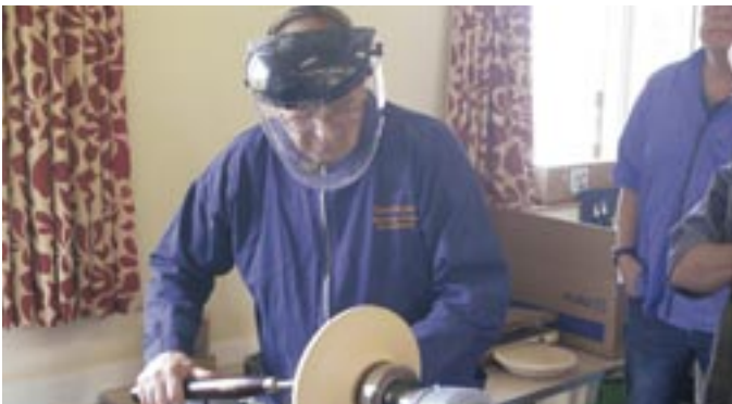
It is important to protect your eyes and face in all aspects of turning by wearing a helmet or face visor and if dust extraction is unavailable it is advisable not to "dry sand". By applying an oil or paste which is readily available, it was used throughout this training day, making the particle's fall to the floor and not become airborne.
