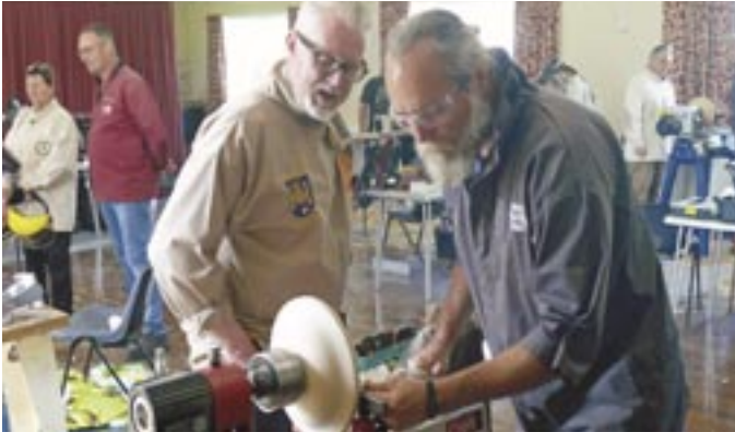
Darren assisting on the tool angle when creating the bowl. The incorrect angle can cause a "catch" particularly when using a push cut.
