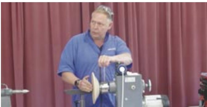
Simon showing where and how the chucking points should be to hold the piece, for hollowing the centre. At this point the bowl blank was held by a screw chuck.
