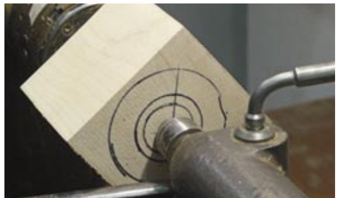
Shaping a spigot to fit the bowl base was the next challenge.
