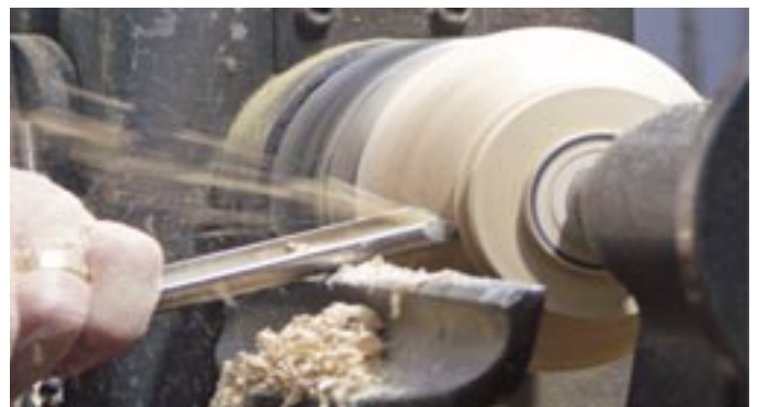
The spigot was cut to size to fit the bowl, and some of the waste removed.
