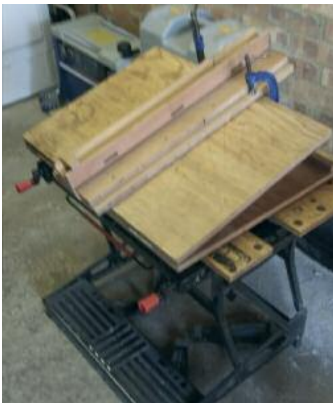
Fig.5. "V" Cradle on Sloping Board used when drilling Stretcher Sockets in the Legs
