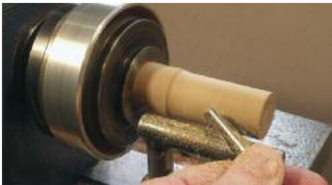
R14. Turning the bullet blank to 22mm diameter.
