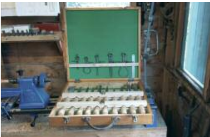
Fig.2. Ashley Iles Turning Tool Set in modified Carrying Case. (It was previously a case for 18" diameter Circular Saw Blades)
