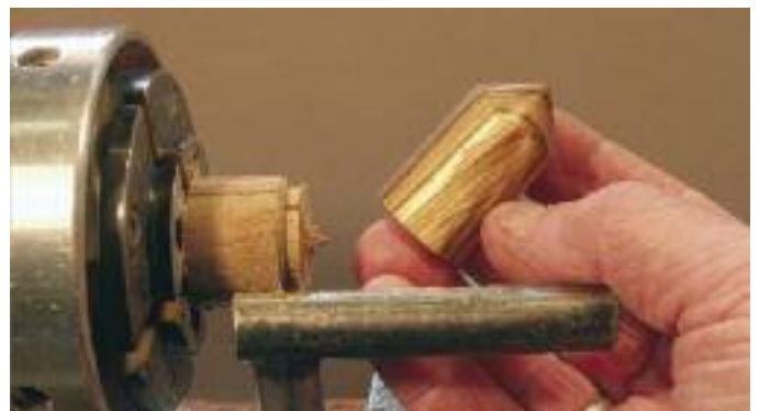
R19. The completed bullet shaped plug.
