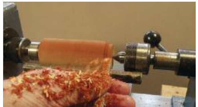
R04. Turning the small tenon at the tailstock end.
