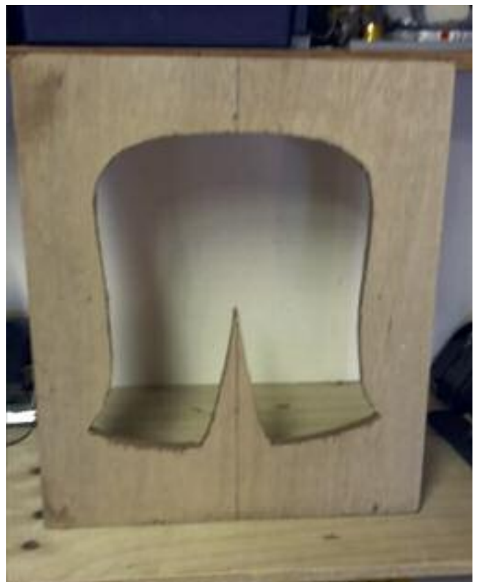
Fig.3. Template used when routing out the Seat Saddle
