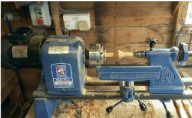
Fig.1. Record Coronet No.2 Lathe with part-turned Cone (2016) Note: I changed the No-Volt-Release (NVR) Switch for a Direct-on-Line (DOL) Starter to provide overload protection for the Lathes Motor.
