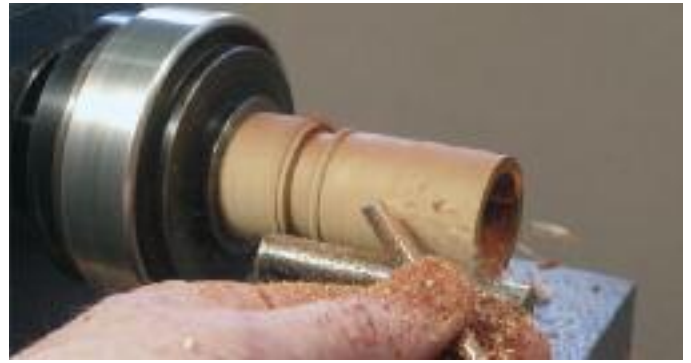
R09. Turning 1mm off the blank.
