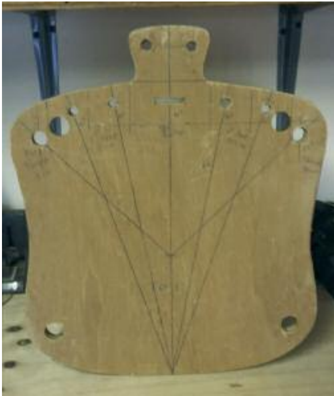
Fig.4. Template used when routing the Seat profile and drilling the Seat Sockets
