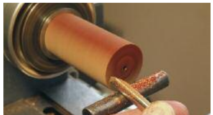
R05. Facing the end of the blank.
