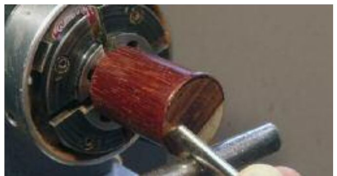
R13. Lightly turning the underside.
