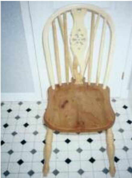
Fig.6. Bow-back made from Ash & Elm (1996) Note: The "wild" grain pattern of the Elm Seat.
