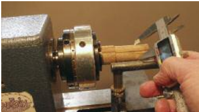
R15. Checking the diameter of the bullet blank.
