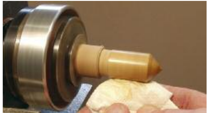
R17. Sanding and polishing the bullet plug.
