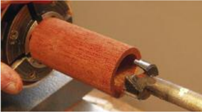
R06. Drill to a depth of 35mm.
