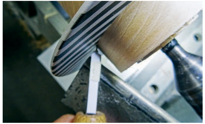
4. micro parting tool cutting
