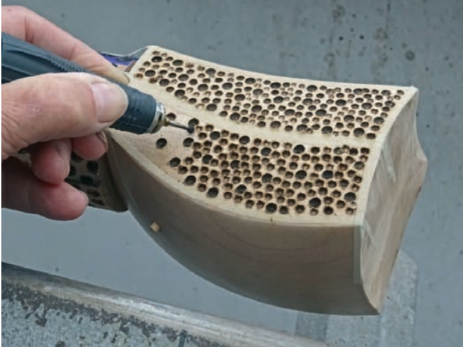
11. Texturing with micromotor burr
