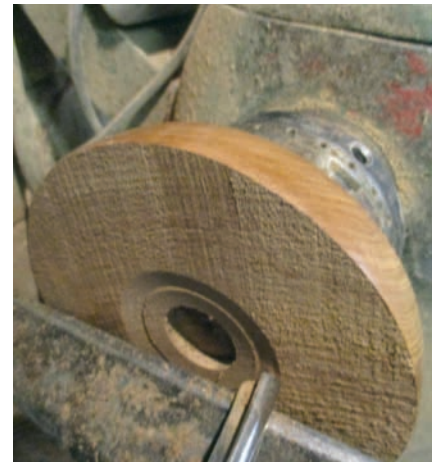
Starting the inside
