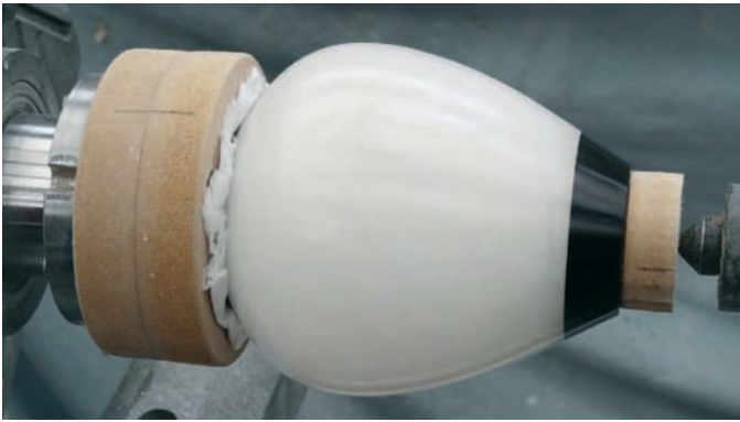
13. Finish shaping of the base
