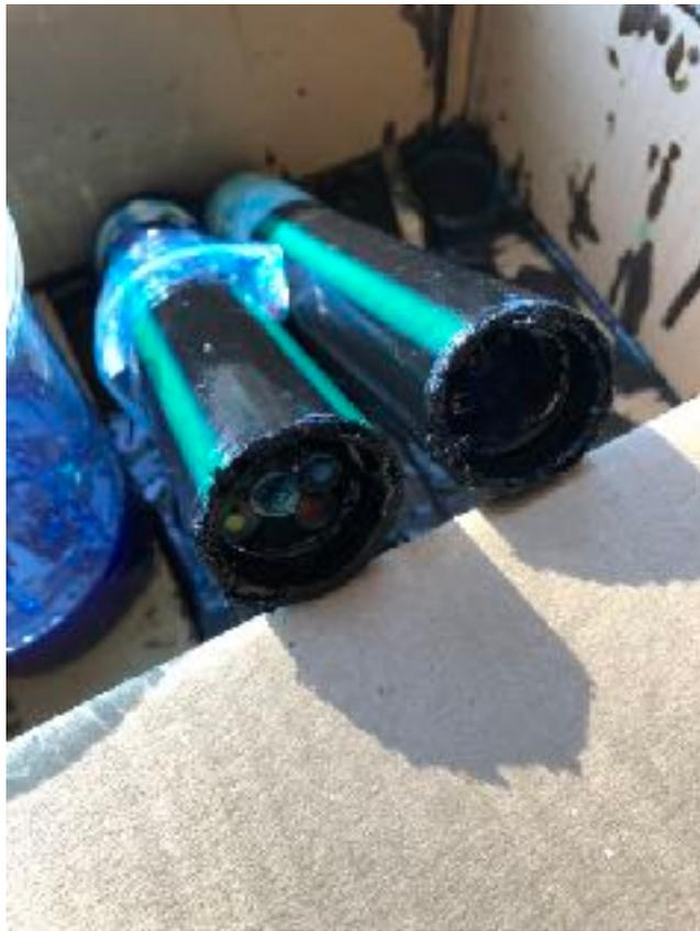
The pipe is sacrificial - although the polyester indeed does not stick to it it is in practice not possible to slide it off without cutting the tube along its length (I used a surform to do this), and even then it requires care.
