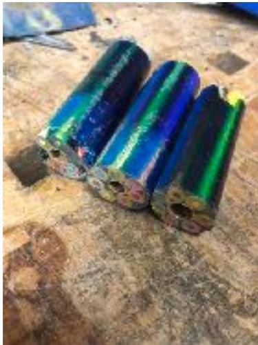
The resin rod is then sawn and sanded to expose the ends of the brass tubes - a pencil is twice as long as the pen tube so I made pairs. The ends of the brass tubes and the joint between them are sealed with a single layer of masking tape, some of which is left in the structure.
