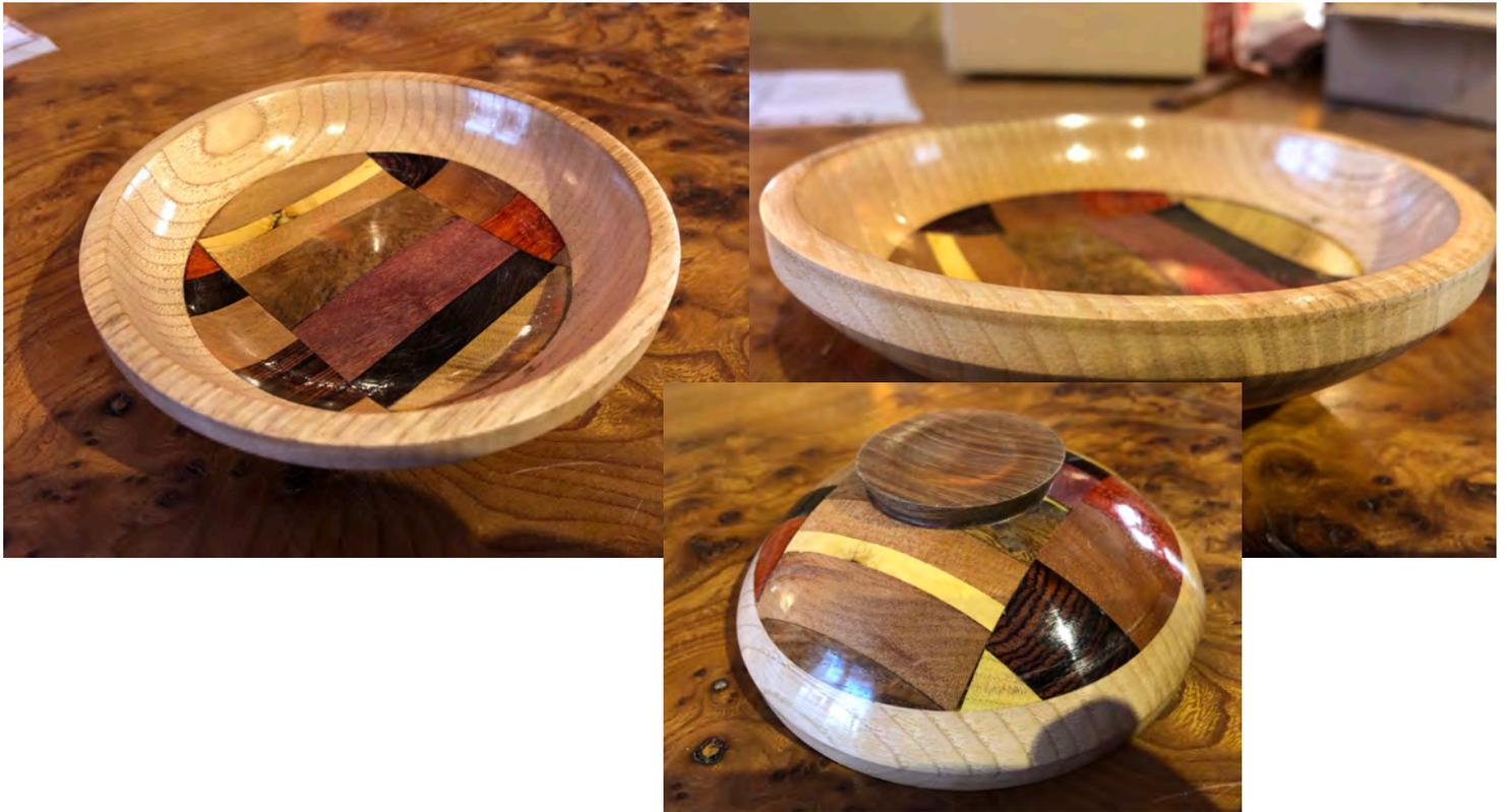
Something else to do with all those little scraps of nice wood too small even for pens! Mostly they are, or can be made, to have two parallel faces so I glued them in strips and cut and refinished with a disk sander (plate on the lathe). Top & bottom also leftovers if slightly bigger.
