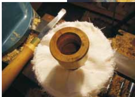
Showing the interior of the pigtail threaded to fit the spindle
