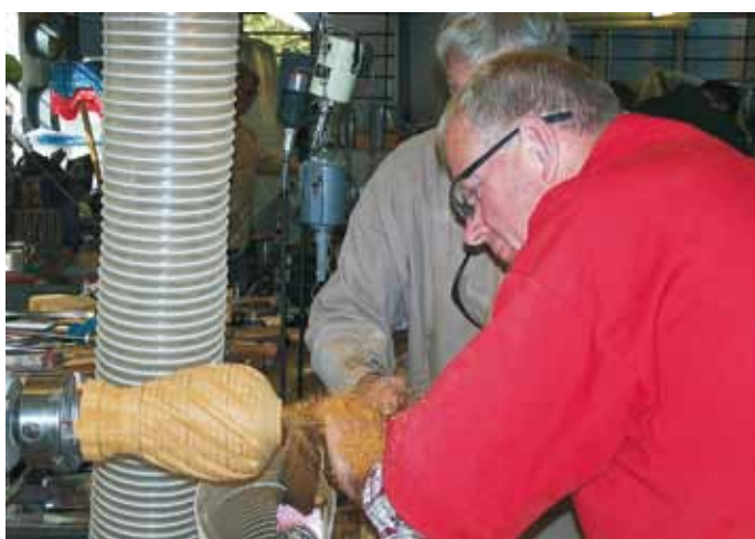
Graham Barnard hollowing out, after using an Arbortech to carve out the voids
