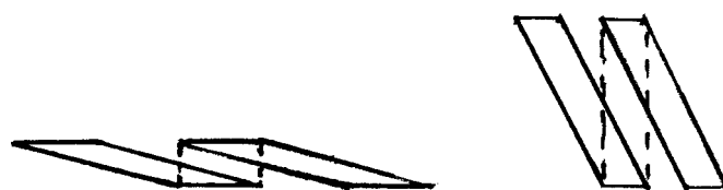
Dia. 3 - The lower the angle, the thinner the blank
