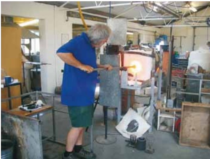
Reheating the glass preparatory to the 'blow'
