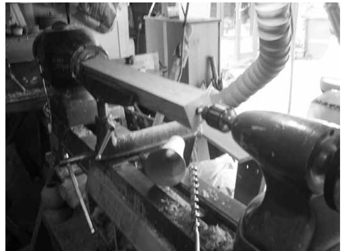
Drilling partway with the short bit
