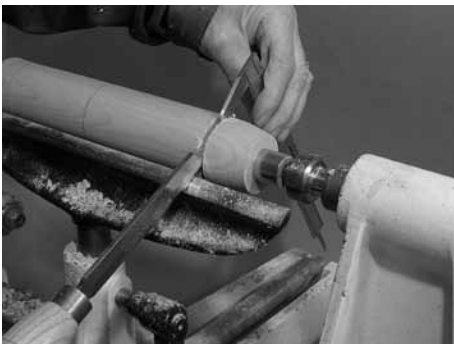
Pic 16 With the ferrule tapped into place remount the blank and with the parting tool and calipers cut the major diameters along the length.
