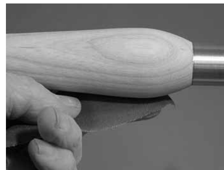
Pic 21 Sand down to 400 grit to give a very smooth finish.
