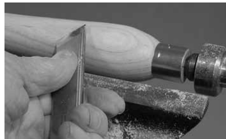
Pic 20 Give a fine cut with the skew chisel to give a fine surface. USE THE BODY.
