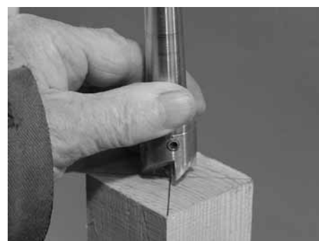
Pic 8 Tap the drive centre into one end with a mallet (do not use a steel hammer).
