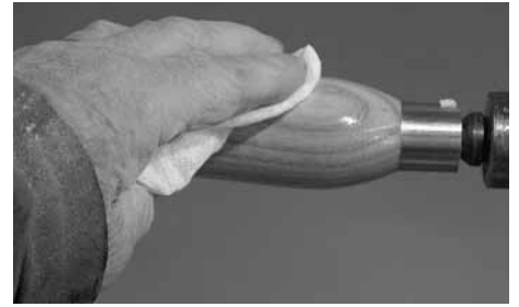
Pic 22 I like to use two coats of finishing oil for the complete handle.
