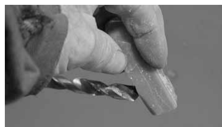
Pic 10 Bring the drill out to clear the swarf and if hot, lubricate with a quick touch of Carnuba wax to prevent binding.
