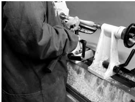
Pic 19 Make your body rise to bring chisel handle up as you cut a smaller and smaller diameter.
