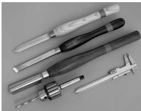
Pic 1 Three chisels are needed, a roughing gouge, parting tool and skew chisel. Plus calipers and a Jacobs chuck.
