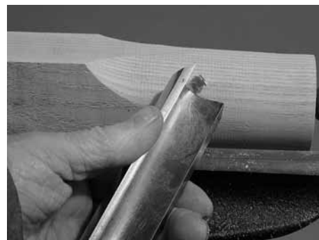
Pic 11 With the blank now mounted between centers turn the square into a round with the roughing gouge.
