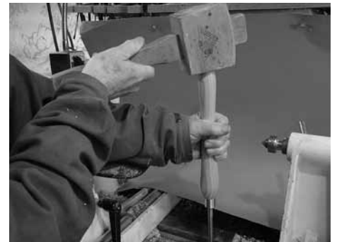
Pic 25 With the chisel end resting on solid wood tap into the handle with a mallet.
