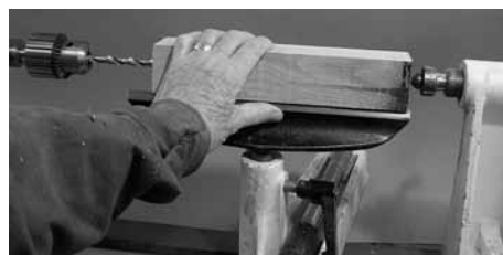
Pic 9 With the 9.5mm drill mounted in the headstock of the lathe, mount the square between the drill and tailstock and using the tool rest to stop any rotation of the square, carefully drill the hole for the chisel. Do not try to put the hole in after the turning.
