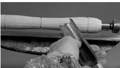
Pic 17 Start to form the rough shape with the roughing gouge using the precut diameters as a guide.
