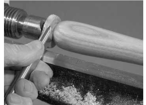
Pic 23 Use the skew chisel to part of the handle which leaves only a small pip to be sanded off.
