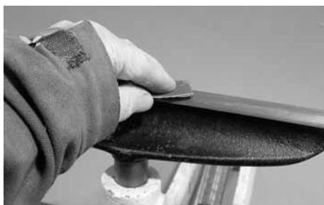
Pic 5 Finish the surface of the rest with 180 grit.
