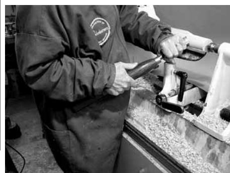
Pic 12 With the tool handle firmly held into the side of the body move the cutting edge along using body movement.
