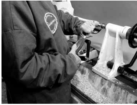
Pic 18 With the tool handle tucked firmly into the body to control the tool, refine the shape working downhill on each cut until the final shape is reached.
