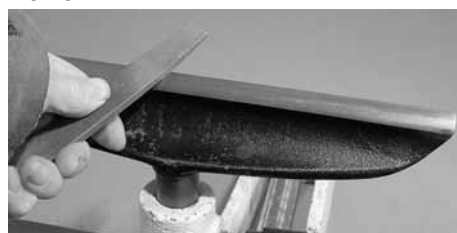
Pic 4 To get really smooth cuts the tool rest must itself be smooth, if necessary use a fine file on it.
