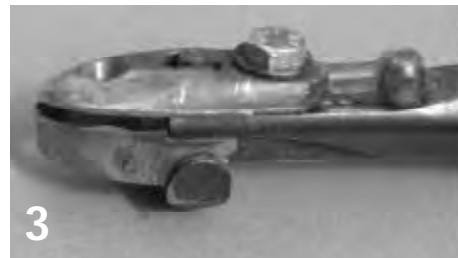
The woodcut tool with a cutting loop protected from being too aggressive with an adjustable hood.
