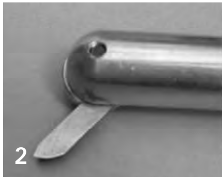
The Sorby small hollowing tool with a little scraping cutter (this is a good tool to start with).
