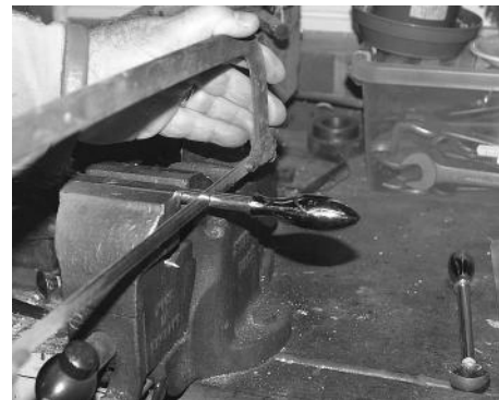
Sawing the bolt insertion to length
