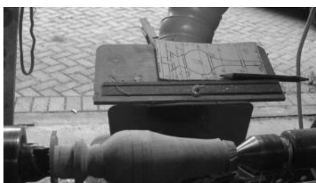
Part turned spindle with template
