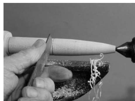
9 – Make a small guide groove to delineate the handle and the blade.
