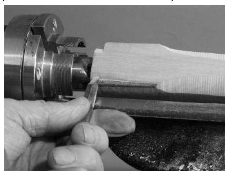
8 – Cut a spigot one end to allow for chucking later. PLANNING
