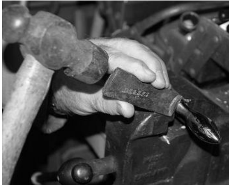
Separating the handle from the shaft
