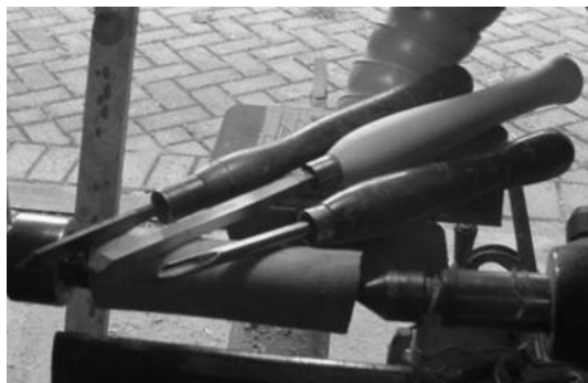
The three main tools used for this work, the Jones Beading Tool is in the centre
