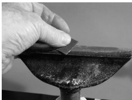
4 – Finish the tool rest off with 180 grit, to get a really smooth surface, this will help your chisels to glide along easily.
