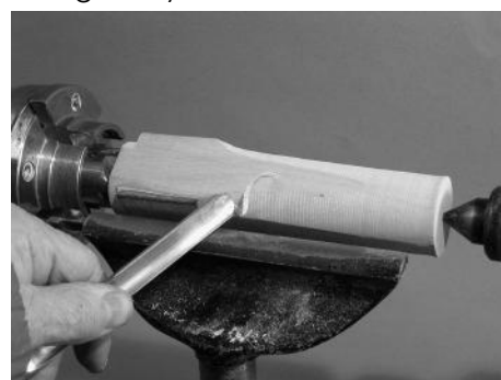
7 – Rough out to the round using the ½" roughing gouge.
