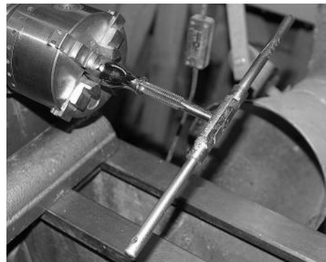
Tapping the 12mm thread in the handle
