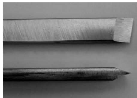
6 13mm skew chisel ground at 15° on both edges. Although larger skews are often favoured, this is the one I use most often, particularly for fine detail. Note the sides of the tool have been rounded slightly to prevent the tool rest getting ridges.
