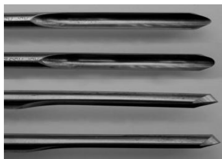
7 10mm basic fingernail gouge ground using the Sorby jig at 30° (the bottom of each pair) this is the main tool used for details on most spindle work. 10mm fingernail gouge ground at 25° (the top of each pair) with smaller radius at the tip. This tool is ideal for very small detail, the tip is equivalent to that of much smaller gouges but the tool has greater stability and is much less likely to vibrate.
