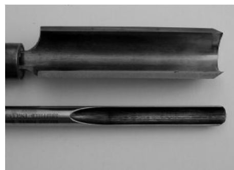
5 35 mm large roughing gouge ground straight across at 30°, this can be used for removing large amounts of wood from spindles and also for finishing cuts on smooth shallow curves. Not suitable for bowls or large diameter logs. 14 mm small roughing gouge ground straight across at 30°, used mainly on small spindles for shallow beads and coves.
