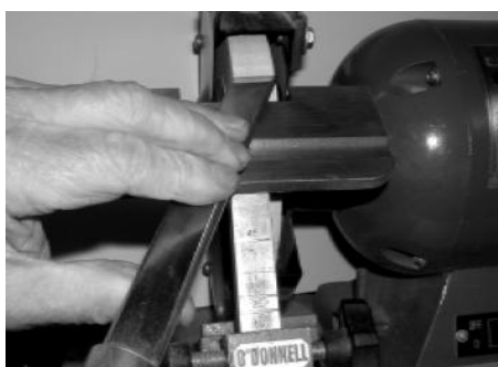
3 A skew chisel being sharpened using the O'Donnell jig set to 15°.
