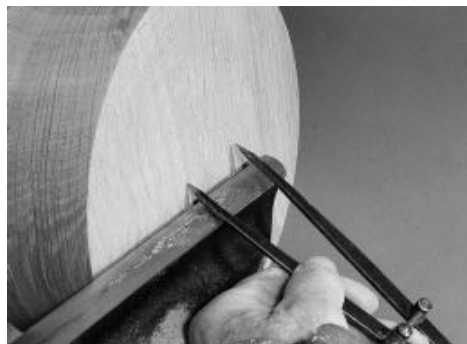
7. Mark the diameter of the spigot which will fit the chuck. Mark with one point of the dividers and check with the other point do not get both points in contact!
