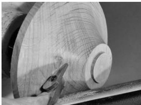
11. Once the shape has been settled and a clean cut managed then use the shear scraper to lightly skim the surface to give a final even finish.
