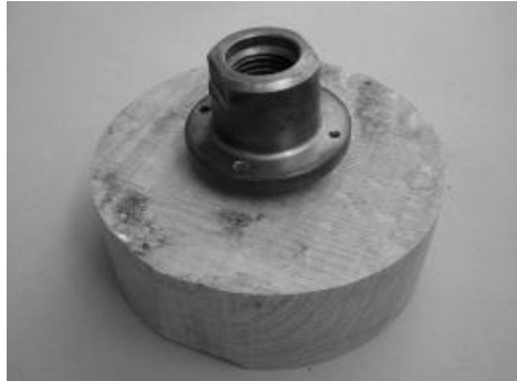
4. Mount the blank on the screw chuck.
