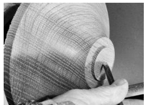
12. Use the point of the parting tool to make a small locating dimple in the centre of the spigot, this will be needed later.
