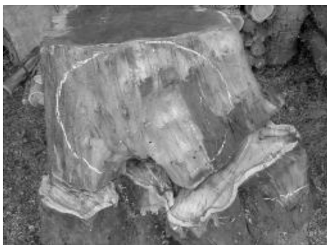
2. First cuts made to obtain the largest possible bowl blank.
