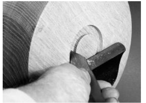
9. Roll the parting tool over to the right and very carefully cut a dovetail on the spigot to suit the chuck.
