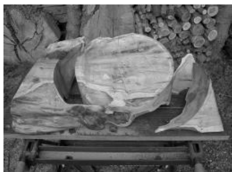
7. Band sawn ready for mounting on faceplate.
