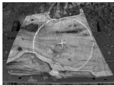
6. Marked out ready to be cut on the band saw.
