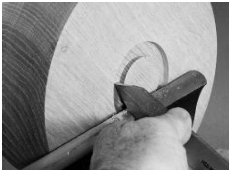
8. Cut a spigot to the correct diameter and depth with the parting tool.
