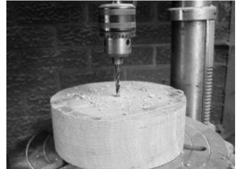
3. Drill a hole for the screw chuck down to the final depth of the bowl as a guide when turning the inside but leave the right amount of thickness remembering the foot and the chucking spigot.
