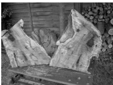
5. .... to reveal the wood grain and colour, The black areas are tree bark which have become encapsulated in the wood as branches have grown together.
