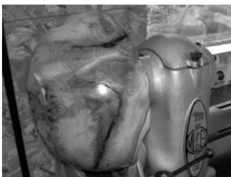
8. Outside of bowl finished and polished ready for re-chucking.
