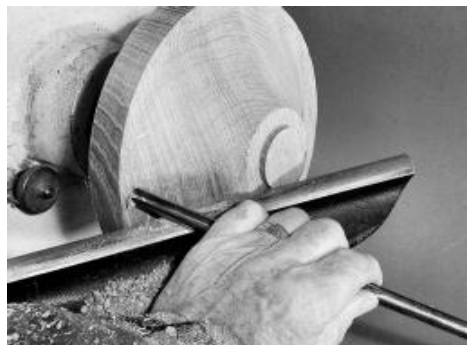
10. Shape the outside of the bowl using a push cut from the outside to the centre, this is with the grain. If you do not get a clean cut check that the bevel is rubbing, re sharpen the gouge if the cut requires significant pressure and always before the final cut.
