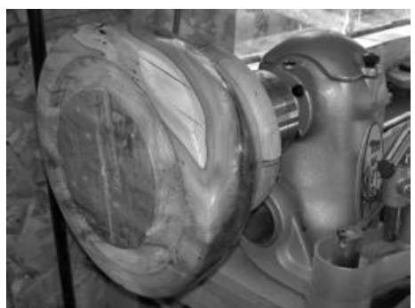
10. Work started hollowing out the inside. Freestanding tool rest had to be constructed due to the large overhang.
