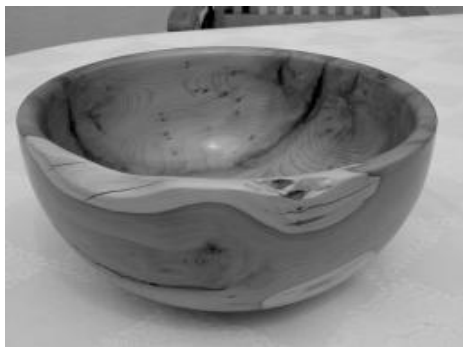
11. Finished bowl showing the lighter coloured sap wood on the rim. Finished bowl is 10 f " Dia. x 4 i" high.
