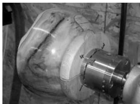
9. Bowl mounted in home made wooden jaws (spigot on this bowl is 4" Dia. These jaws will also take a 6" Dia. spigot).
