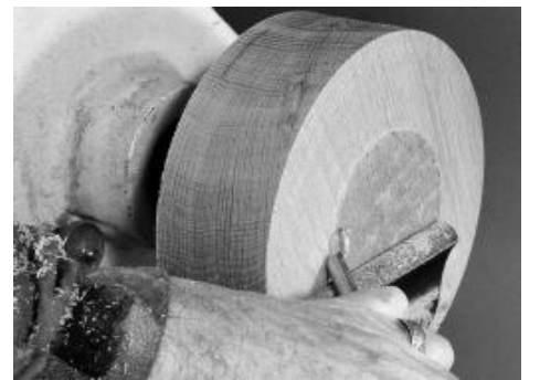
6. Use the bowl gouge to true up the face of the blank, always keep the tool rest as close to the wood as possible.
