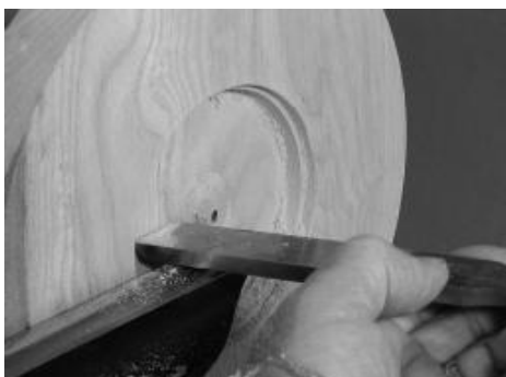
10 Using a flat scraper run across the bottom of the recess to give a flat surface. The back of the clock should now be fully finished as shown for the front later.
