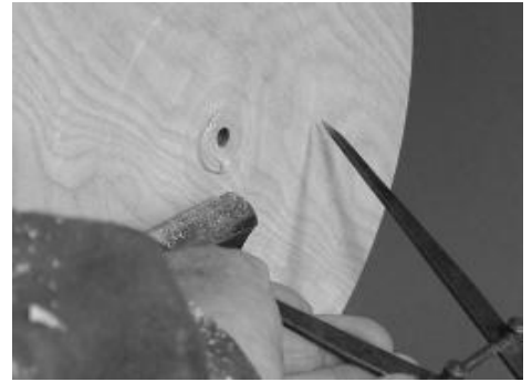
6 The chucking recess is marked using one point of the dividers and checking against the other point. Do not let both points touch the wood or !$%^.
