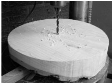
2 The wooden blank being drilled for a screw chuck.
