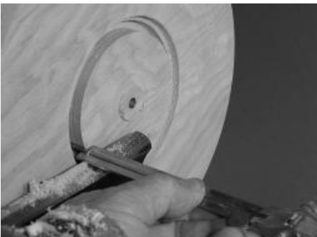
8 Check the depth of the recess to make sure that the clock movement will not protrude.
