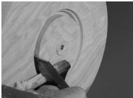
7 Cut in to the back, with the parting tool facing slightly up, to form the chucking recess which also takes the clock mechanism. Make a similar groove near the centre taking care not to catch the screw chuck.
