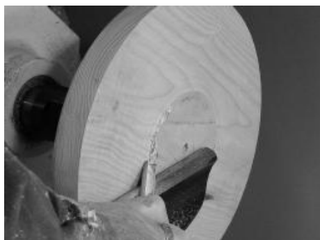
11 Reverse the blank on to the 4jaw chuck checking that it is running true and face off the front. There will be problems with fixing the numbers if this face is not very flat.
