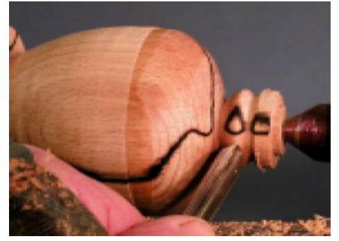
15 Finally shape the lid using the bottom as a jam chuck.
