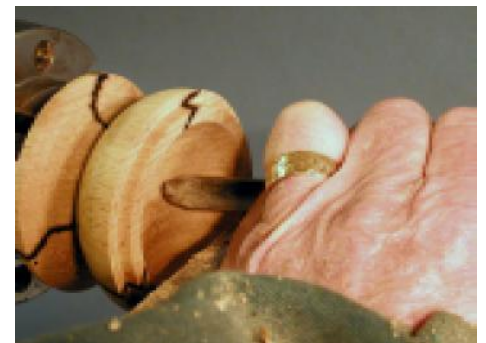
9 Rough hollow the inside of the lid and clean up the inside edge.
