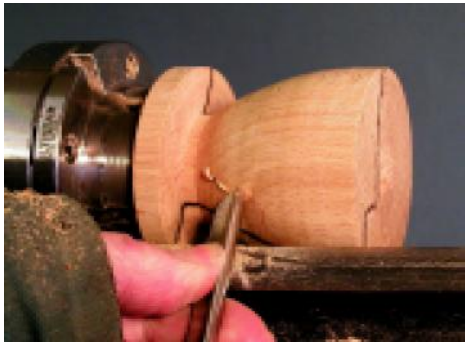
13 Next mount the bottom of the box on the chuck and rough shape the outside.
