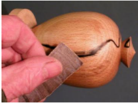
16 With the top and bottom blended together sand the whole of the outside of the box, finish with melamine and buff.
