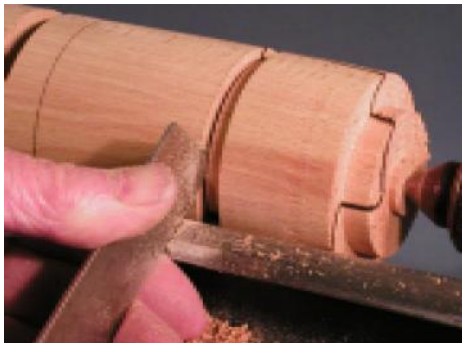
7 Part off the lid from the base using a thin parting tool so that very little wood is lost and grain will still match (very curly figure will be difficult to match).
