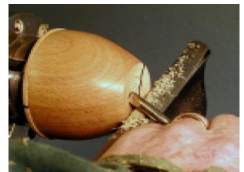
21 Two little decorative rings are cut in the bottom to show that you care about it using the little round chisel. (an normal skew or the tip of a parting tool can be used)
