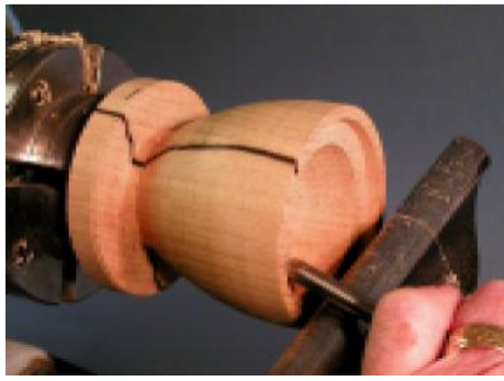
14 Rough out the inside, and using the little straight chisel pointing slightly up, cut a tightly fitting recess for the lid.
