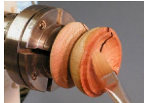
12 Apply a good coat of melamine and buff to a sheen.
