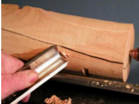
5 Mount the wood between centres and rough down to a cylinder.
