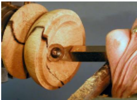
10 Finish the inside using shear scraper (the Sorby tool is ideal for this) an alternative is to use a standard round ended scraper.
