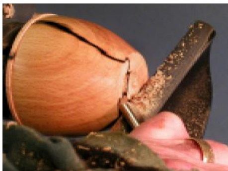
20 Reverse the box onto the jam chuck and refine the bottom, making sure that it is concave (if convex it will rock).
