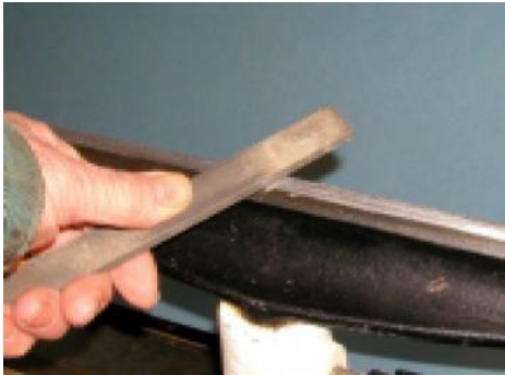
4 Before starting to turn it is worth checking the toolrest and giving it a smooth down with a fine file if there are any nicks in it.
