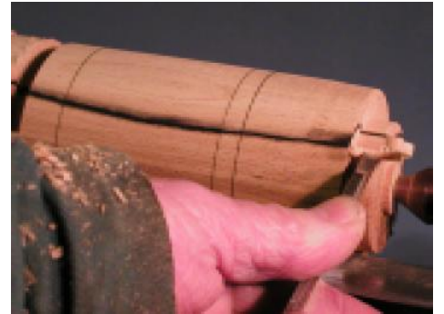
6 Mark out the lid and base and cut a spigot at each end to fit in the chuck.
