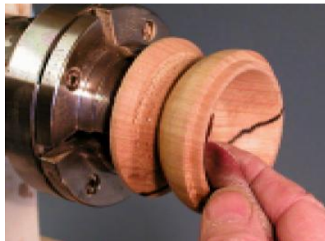
11 The finish left by the shear scraper makes sanding easy, starting with 240 grit working up to 1200 grit..
