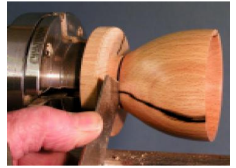
18 The bottom may now be parted off using the thin parting tool.
