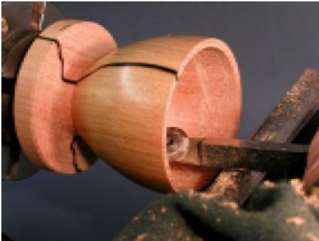
17 Take the lid off and refine the inside of the box using the shear scraper, sand and finish.
