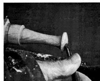
Cut the domed top with the spindle gouge before thinning down the base
