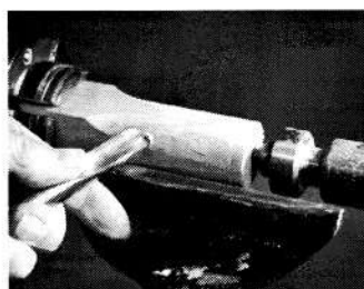
Blank gripped in chuck jaws and roughed down to the right diameter
