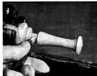
The base of the peg can now be reduced to the correct size
