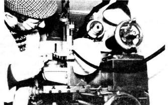
in a flexible drive shaft which is fixed into a slide table. It is a strange experience watching patterns cut without the item flying round, it needs to be seen!
