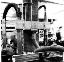
with the help of solvent cement and some geometry you thought you had forgotten. I use 4" flexible ducting to the combined hood/guard of the saw-bench and for the wandering hose which makes it easy to clean the floor and so reduce dust build-up. The main duct and branch to the lathe (the most difficult machine to collect from), is 6" diameter.
