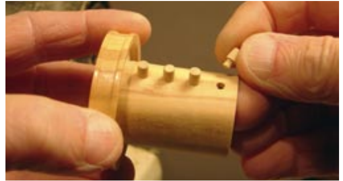
Photo. C40. Glue the bullet shaped pins in place.
