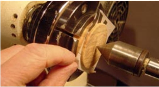
Photo. C36. The locking ring blank is held on a 'newspaper/glue' chuck.
