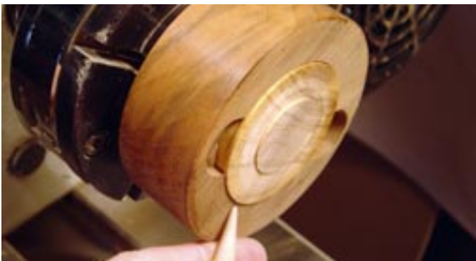
Photo. C18. Note the finger holes allowing the ring blank to be released.
