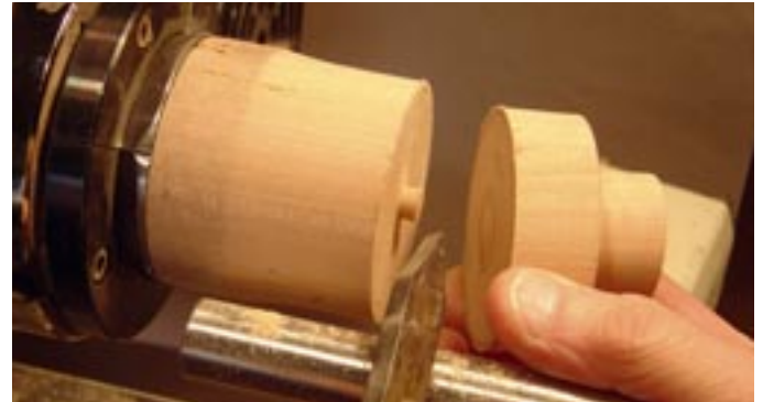
Photo. C1. Turning the supporting plug.
