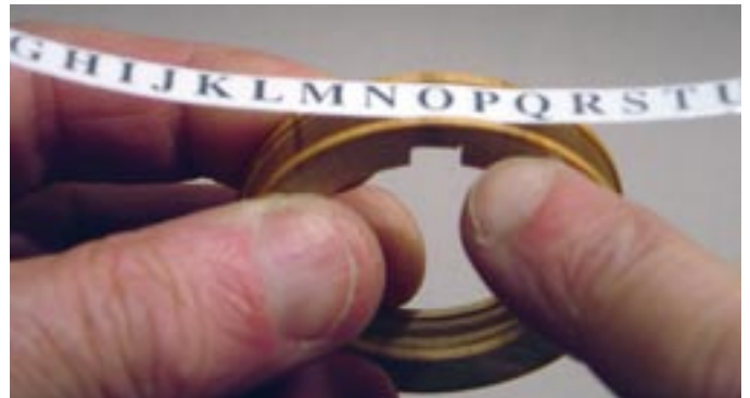
Photo. C47. In my example the letter O is fixed opposite the slot in one of the rings.
