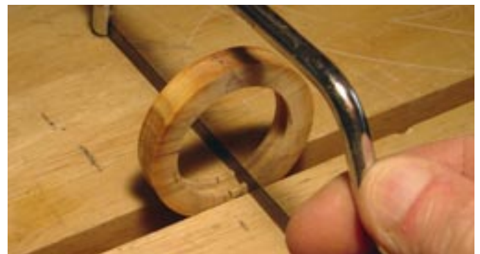
Photo. C41. With great care saw the slots in the rings.
