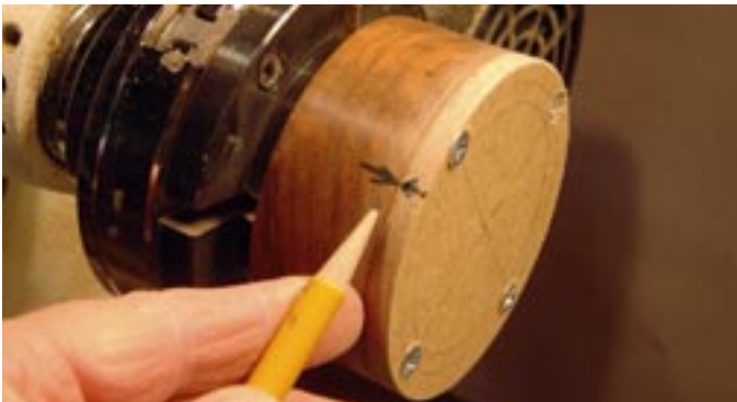
Photo. C19. Note the datum on the collar and on the 'chuck' body.
