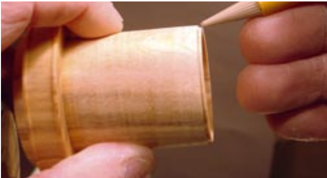
Photo. C29 & 30. The step is turned upon which the locking collar will fit.
