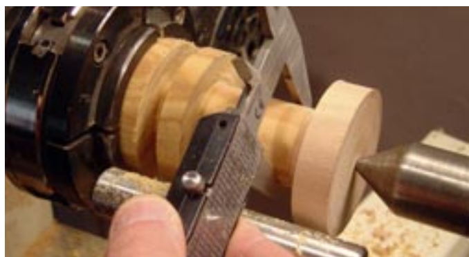
Photo. C6. ....to [1 \frac{3}{16} in] 3cm diameter.
