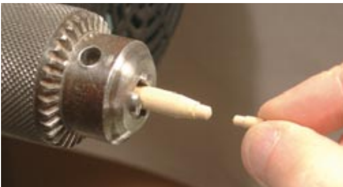
Photo. C39. Turning the bullet shaped pins.
