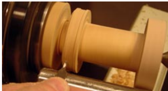
Photo. C7. Turning the 'recess' in the top rim.
