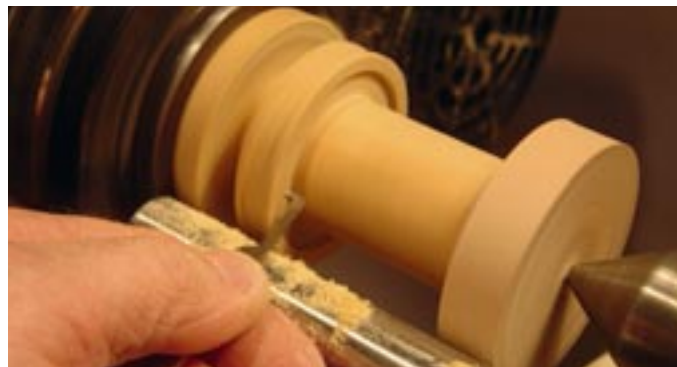
Photo. C8 & C9. Undercutting beneath line Y.
