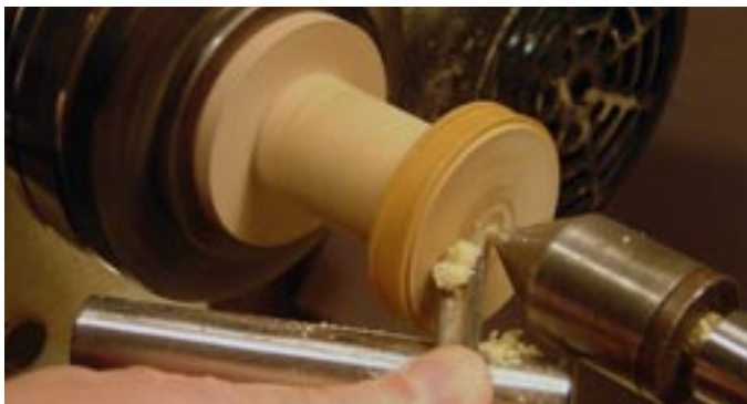
Photo. C11. Support the base whilst partially turning the end flat.
