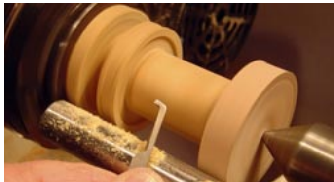
Photo. C8 & C9. Undercutting beneath line Y.
