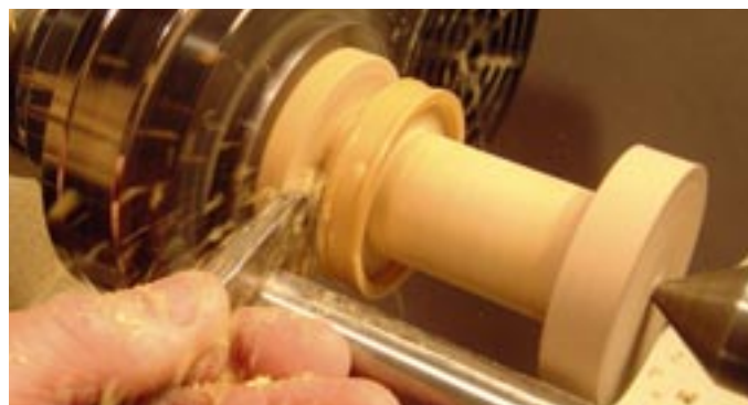
Photo. C10. Part off on the headstock side of line X.
