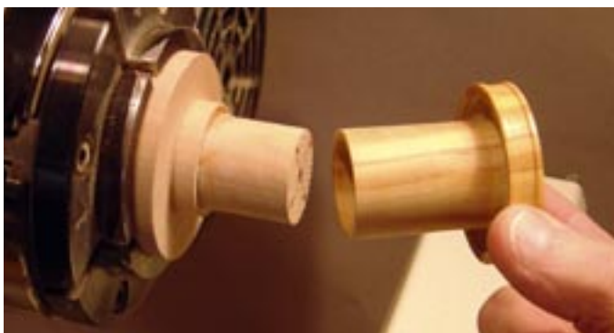
Photo. C13. Loosen the hot melt glue to release the work from the supporting plug.
