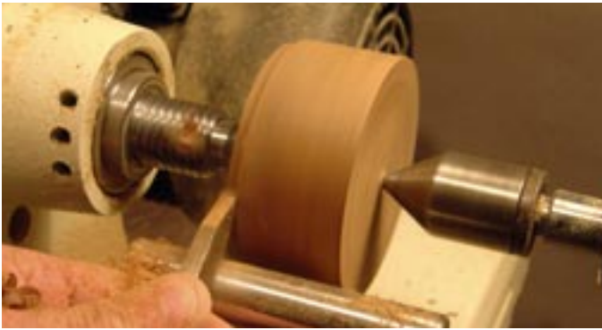
Photo. C16. Preparing the 'chuck' to hold the rings.
