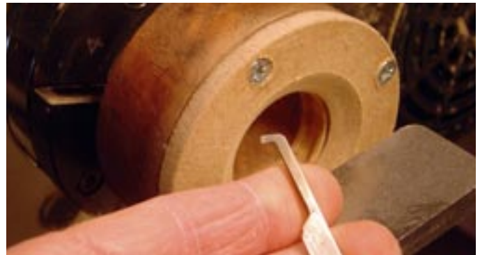
Photo. C22. Turning the undercut in the rings with the specially shaped tool.
