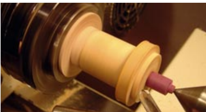
Photo. C32. Temporarily hot melt glue the 'top' to the supporting plug.
