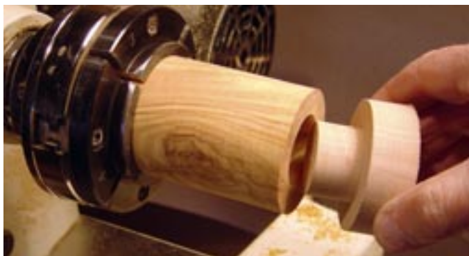
Remove the drill and fit the prepared plug into the drilled hole. Bring the centre up for support. [Photo. C25]
