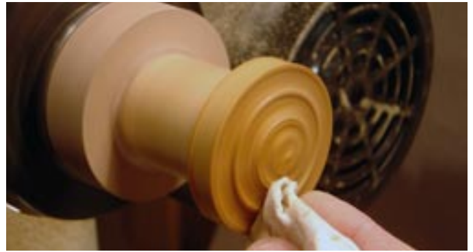
Photo. C33. When the end has been turned sand and polish.
