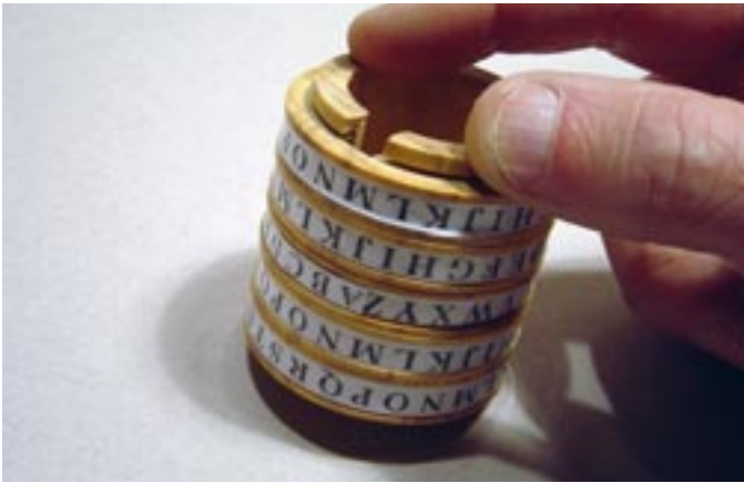
Photo. C49. Finally gluing the locking ring in place.
