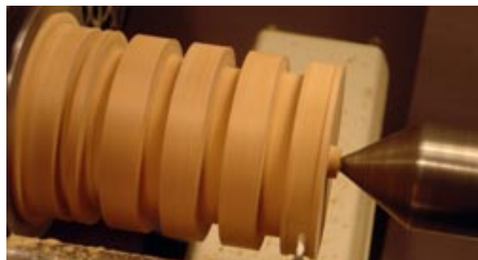
Photo. C14. Turning the recesses on the ring blanks.
