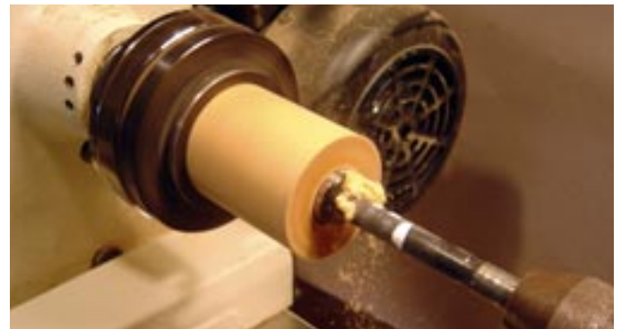
Photo. C2. Drilling into the base blank.
