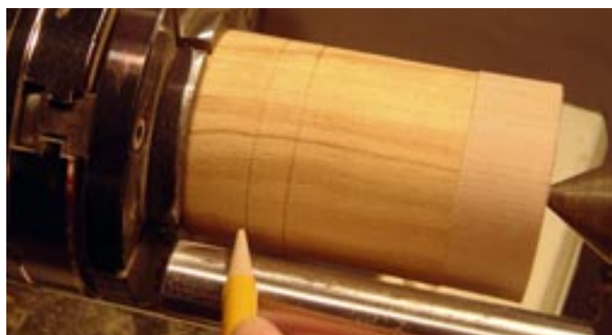
Photo. C4. Locating position Y on the turned blank.
