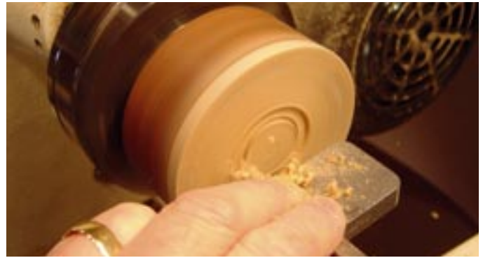
Photo. C20. Turning through the MDF collar and into the void.
