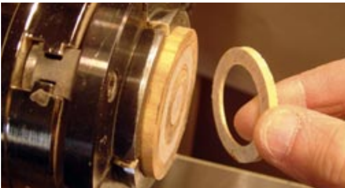
Photo. C38. With great care split the newspaper/glue joint holding the finished locking ring.
