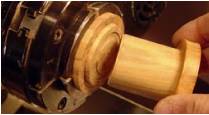
Photo. C37. Test the 'top' recess onto the part turned locking ring.
