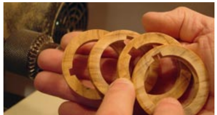
Photo. C42. All 4 rings with slots cut.
