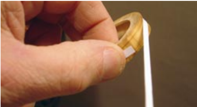
Photo. C44. Check the circumference of the ring recess with a thin strip of paper.
