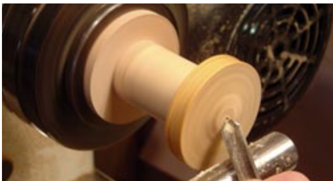
Photo. C12. Finish turning the end face of the base.
