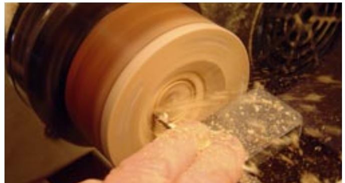
Photo. C21. Turning the inner hollow of the ring blank.
