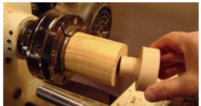
Photo. C3. Fitting the supporting plug.
