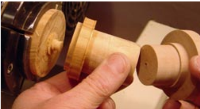
Photo. C31. Parting off the part finished 'top'.
