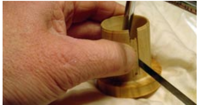
Photo. C34. Cutting the slot in the body of the 'top'.
