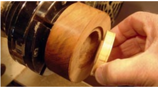
Photo. C17. Checking a ring for fit in the 'chuck'.
