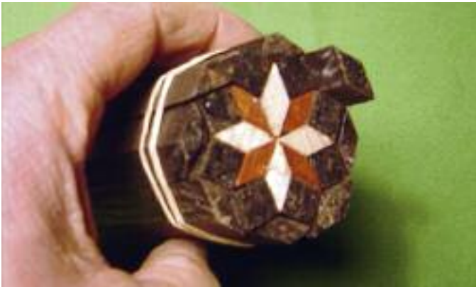
Photo. A17. Gluing the 8 blackwood diamond shaped sticks around the outer edge. lengths being glued together they are prone to 'spring' slightly. Just a few millimetres down the joints will be quite tight. [Photo. A18]
