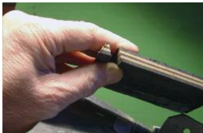
Photo. A26. The laminated blank from which the triangular stick is cut.
