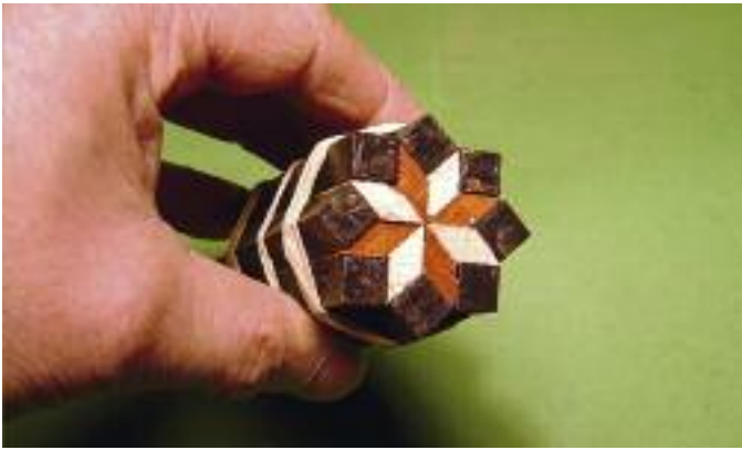
Photo. A16. The glued squares are held with elastic bands whilst the glue dries.
