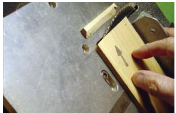
Photo. A2. The first cut to determine the size of the angled face. Note the grain direction.
