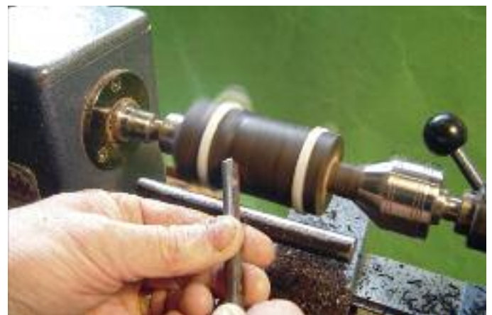
Photo. A21. Having moved the cable ties the central section can be turned.
