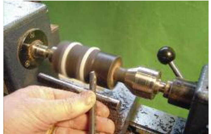
Photo. A20. Turning the blank. Note the cable ties.
