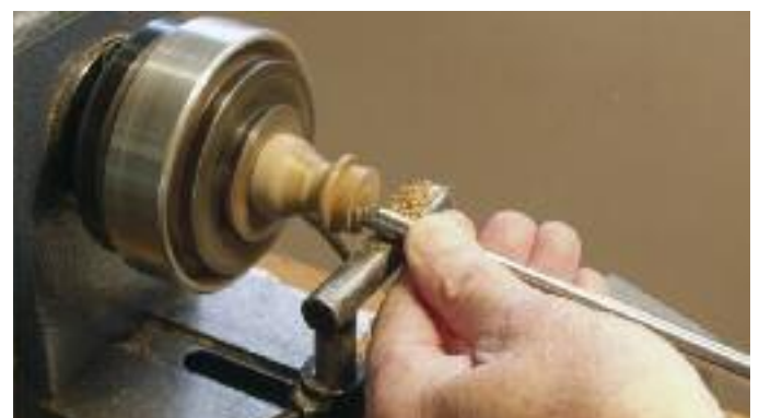
7. Turn the exposed end carefully down to 5mm thick.
