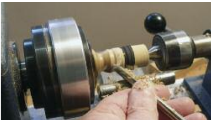
10. Waste wood support at the tailstock end whilst making a sweeping cut with a gouge.
