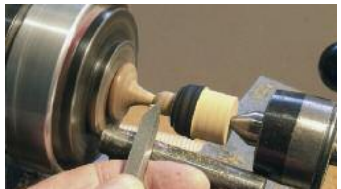
14. Carefully round over one edge of the 9mm diameter top.
