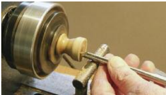
9. With light cuts turn the end face.
