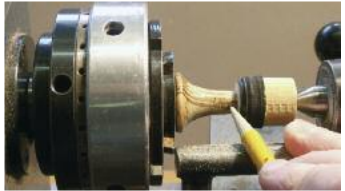
11. The area next to the waste wood support is turned to 9mm diameter.
