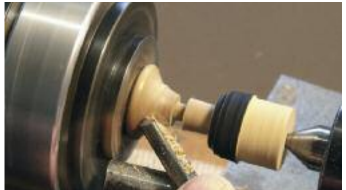
13. Make a sweeping curved cut down to the 3mm diameter section.
