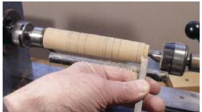
1. Turning the end to 19mm diameter.
