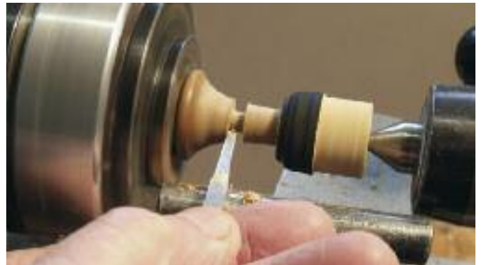
12. 9mm away from the waste wood support turn down to 3mm diameter.
