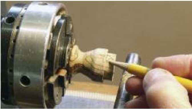
8. Reversed in the lathe. Now cut away the stub tenon shown here.
