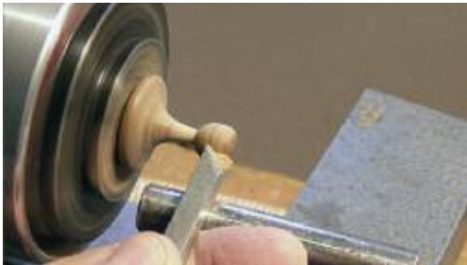
15. Having removed the support the top of the 9mm diameter section can be rounded over.
