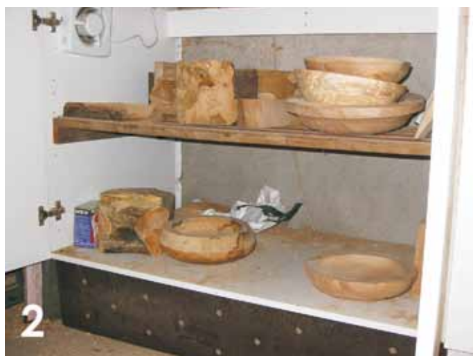
Home-made kiln – I use a kitchen cupboard (in the workshop). It is double width (1000mm) but a smaller one would work well. I have a small extractor fan
