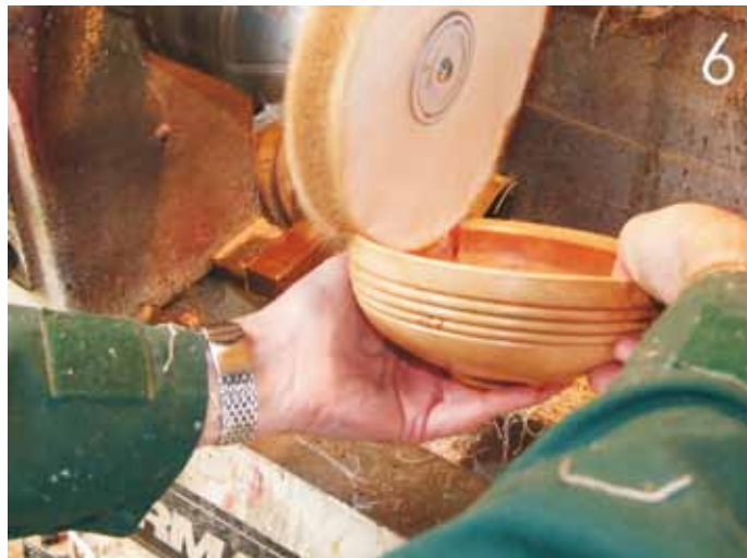
Photo 6 - Based on that experience I decided to polish the rest of the rim in this direction instead. I'm pleased to say the bowl was undamaged and the lesson well and truly learned. This was the only occasion that anything felt out of my control.
