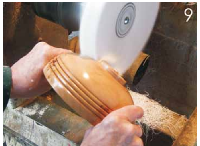
Photo 9 - But the final mop (C), hand-in-hand with the carnauba wax stick, really put the depth into the shine. If following in my wake, be careful not to overload the mop with carnauba, otherwise unsightly-and-hard-to-remove waxy lines will be deposited onto the work piece.
