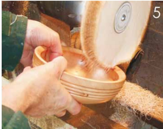
Photo 5 - Immediately after taking this shot of me polishing the rim the mop quite rudely snatched the bowl from my hands and threw it ignominiously against the wall. Hmmmm, sharp edges at right angles to spinning cotton, another good reason to keep the lathe speed down.
