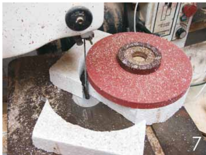
Photo 7 - A quick whip around with the band saw removes the excess polystyrene.
