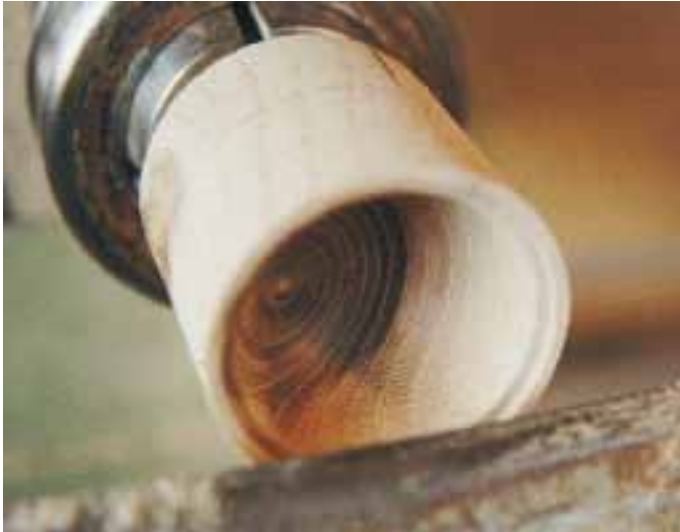
A lip is cut for the top to sit on
