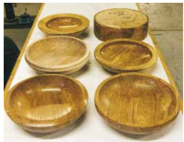
The five almost finished bowls with a bowl blank (back right) that was the starting point of each bowl.
