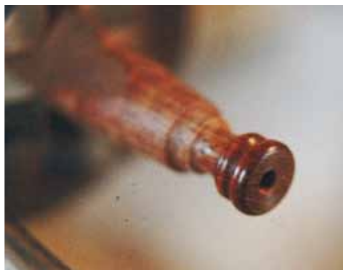
The turned beads at the base of the finial
