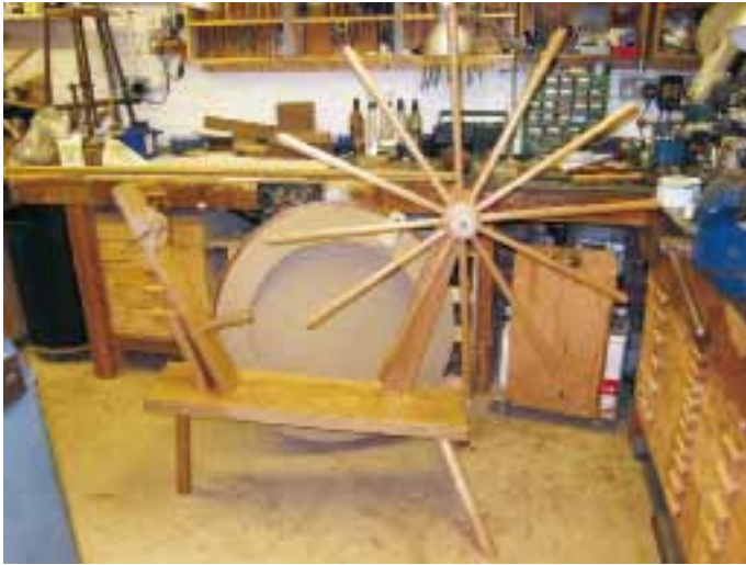
3 - Great wheel under construction (rim hoop bending jig behind)
