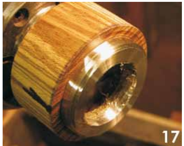
17. The next task nearly went very, very wrong! I screwed the bottom into the top and proceeded to cut the shoulder and face off the front which all went well as you can see. Then I tried to unscrew it. I thought it had just expanded at first and then realised it was more serious, it was stuck. The forces of turning had locked it together. I had to very carefully fix my mole grips onto it to get enough leverage to release it. Fortunately it worked. Next time I'll put a slip of paper or thin card in between the two to stop that happening.
