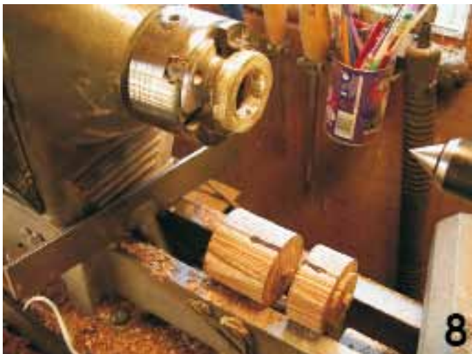
8. I put the insert straight into the chuck jaws ready for turning. You can also see the prepared box blank as well.
