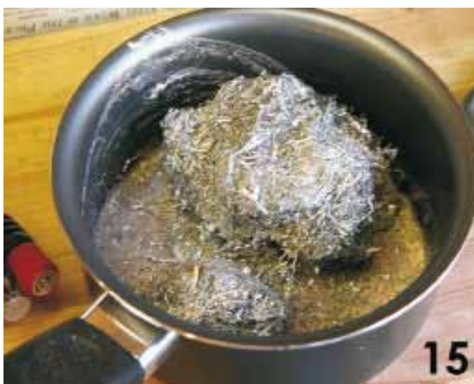
15. All the swarf and the remains of the pewter (lots!) in the pan ready for next time.
