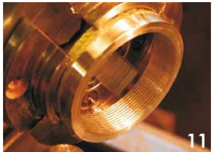
11. Here's the result. Polish with 0000 wire wool.
