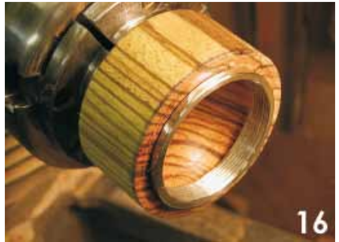
16. I turned out the lid and fitted the ring. I used medium superglue, I would have used the thick stuff but I didn't have any. Then I ran some thin around the join at the back of the ring. A quick spray with accelerator and I was able to skim off the face and edge and cut a small chamfer on the edge. Looks like a whisper of swarf there which I took away afterwards.
