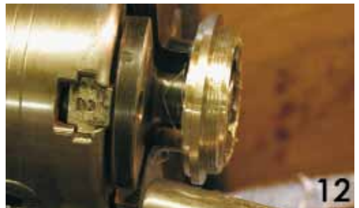
12. I mounted the other piece, trimmed it up and chased the male thread as per usual. One handy thing with pewter is, if you need to reduce the diameter and re-cut the thread you don't have to change the speed, it cuts fine at 350 – 450 rpm.
