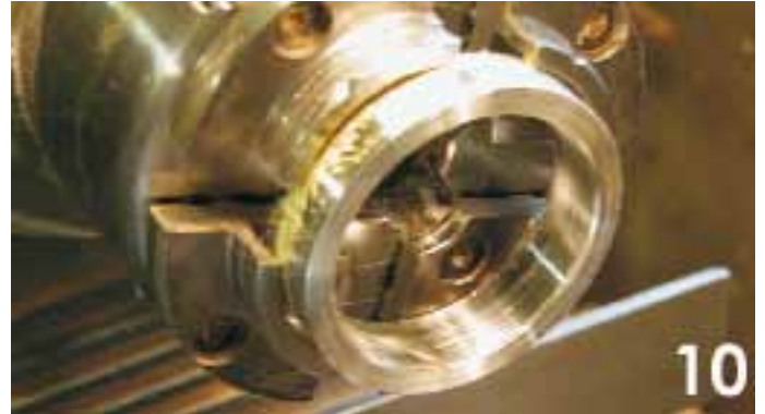
10. Here it is ready for the female thread to be chased. I did this in exactly the same way as I would for wood.
