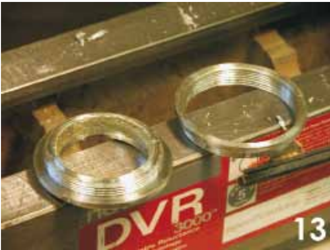
13. Once the male threads were cut I fitted the female and cut the shoulder. Cutting makes them quite hot, you have to let them cool down before they will separate. Here are the two pieces.
