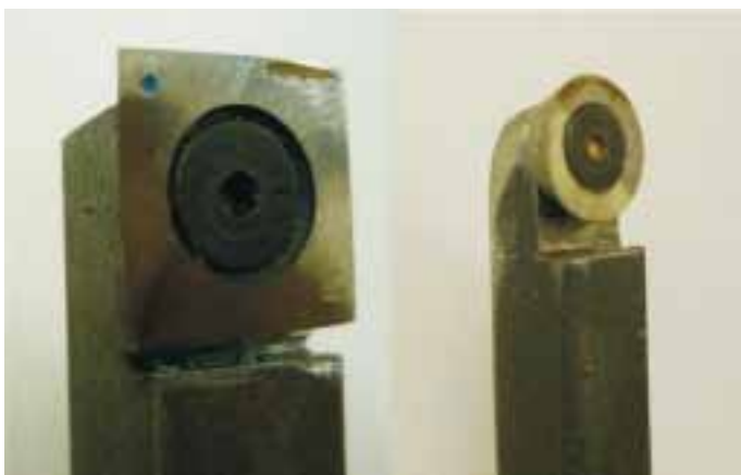
Bill's carbide tips in their homemade holders
